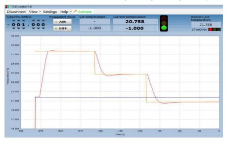
Fig.2. Main window of TCB Control program
