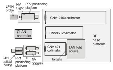
Fig.2. Block diagram of the NVS test station
