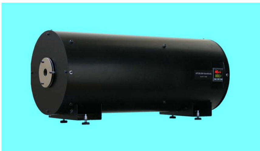
Fig. 1. Photo of the HTCB-25D-1200 blackbody
