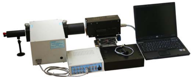
Fig.4. Photo of FT test system in configuration for measurement of spectral parameters (FT-S configuration)
